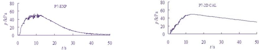
Fig.5 Response of pore pressure gauge P7 in test and calculation during earthquake
