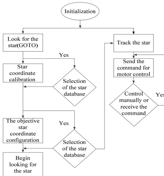
Fig. 3 Telescope Control Program Flow Chat
