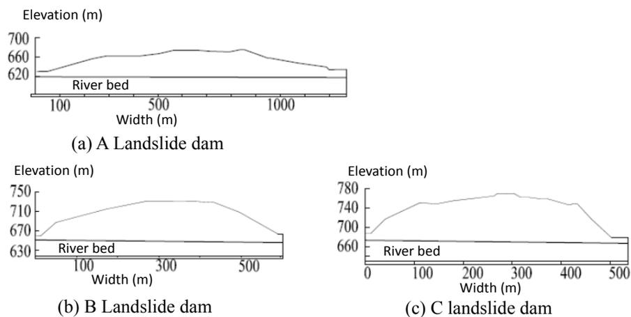
**Fig. 5.** Typical cross sections of landslide dams: (a) soil-type; (b) rock-soil mixture type; and (c) rock-type.
