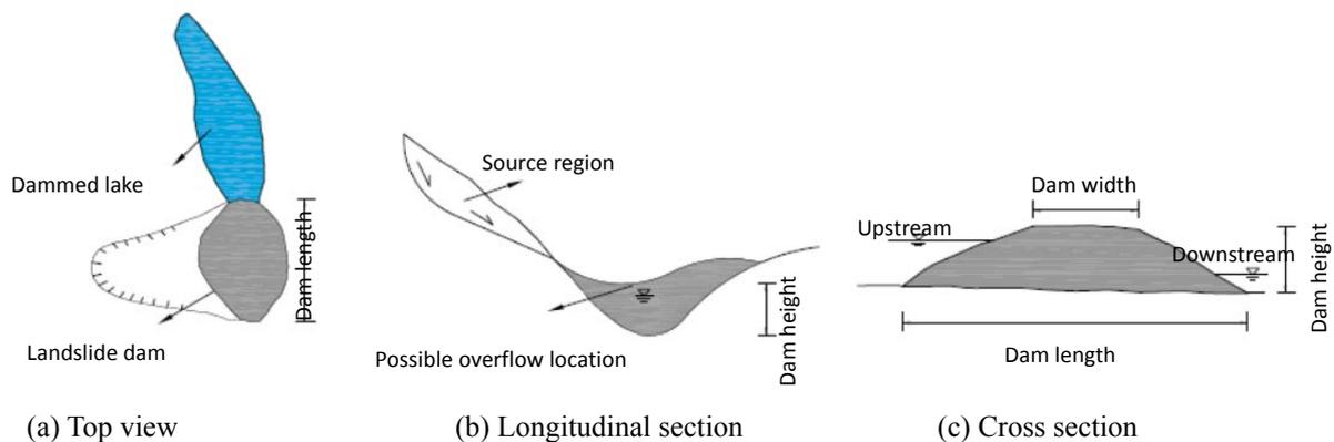
**Fig. 4.** Sketch of geomorphometric properties of a landslide dam.
