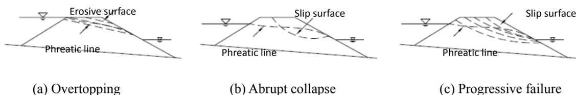
**Fig. 7.** Three types of collapse of a landslide dam.
