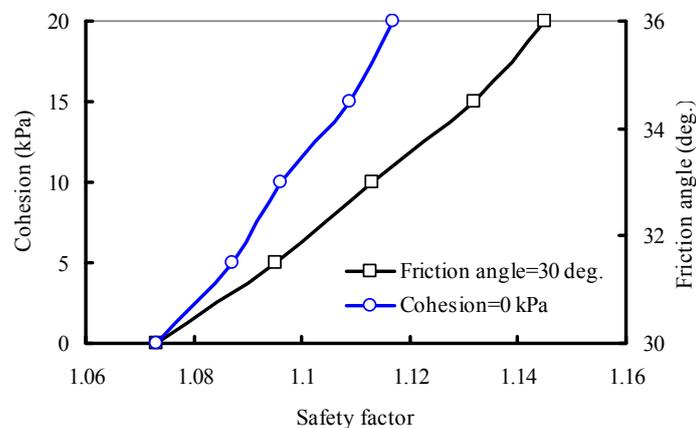
Fig. 8. Results of sensitivity analysis of shear strength impact on stability of a landslide dam.
