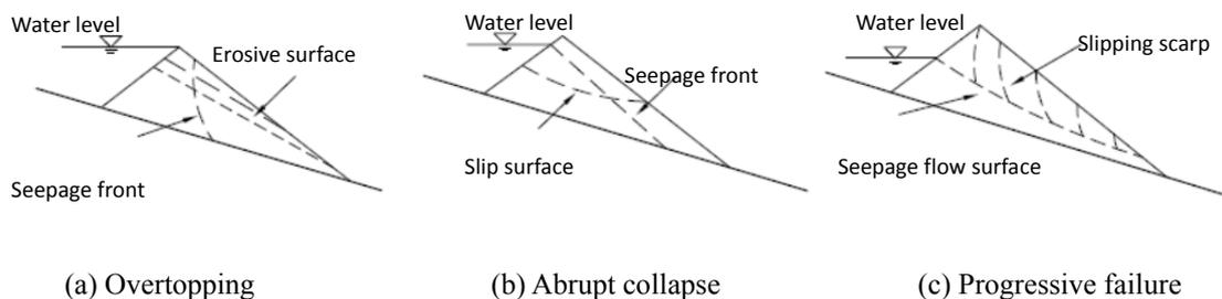
**Fig. 6.** Failure modes of landslide dams (modified from Takahashi and Nakagawa 1994).
