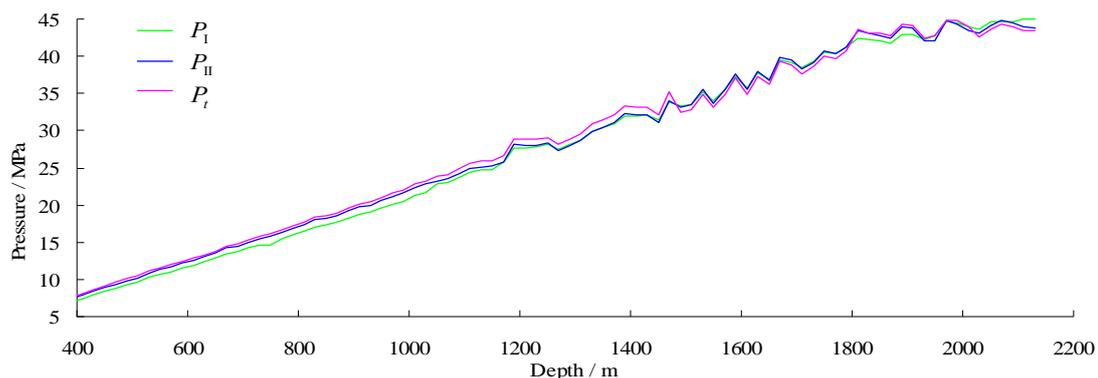
**Fig. 7.** Fracturing pressure of Well-A.
