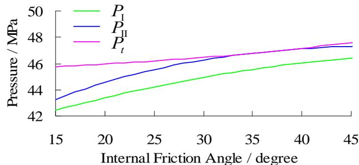
Fig. 6. The influence of internal friction angle on fracturing pressure.
