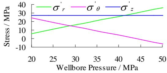
**Fig. 1.** Variation of principal stress with wellbore pressure at maximum horizontal stress direction.
