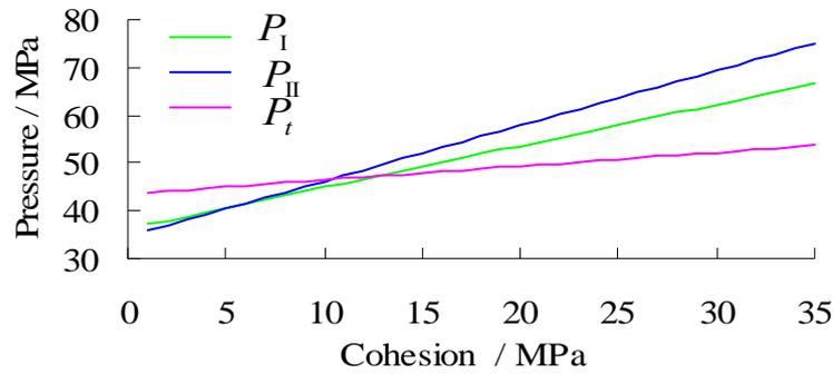
Fig. 5. The influence of cohesion on fracturing pressure.
