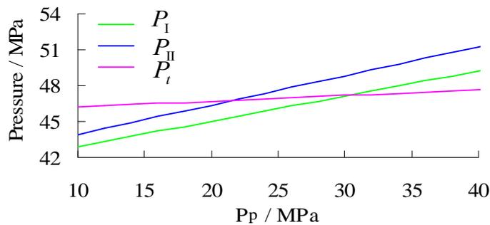
**Fig. 4.** The influence of pore pressure on fracturing pressure.
