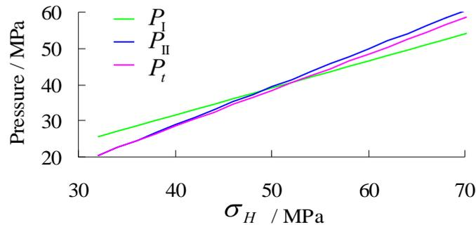
Fig. 2. The influence of in-situ stress magnitude on fracturing pressure.
