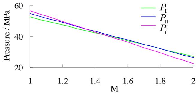
**Fig. 3.** The influence of in-situ stress non-uniformity on fracturing pressure.
