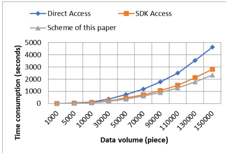
Fig. 4. Time consumption under three different schemes
