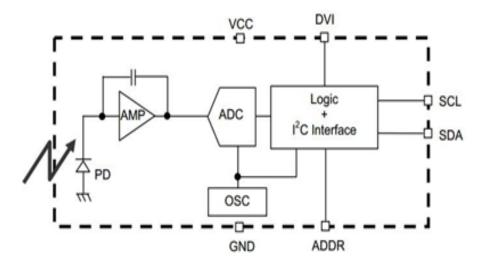
Fig. 6. BH1750FVI circuit diagram
