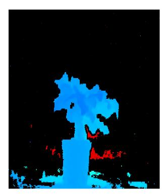
Fig. 4. Three-dimensional image obtained by L515
