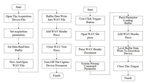
Fig. 10. Flowchart of software design of human-computer interaction interface
